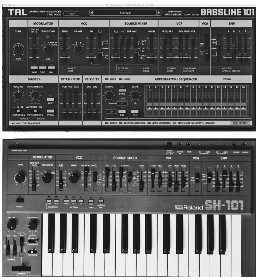
Figure 6.1 Togu Audio Line's Bassline 101 versus a Roland SH101. The “VCF” appears in roughly the same place in both the device interface and the skeuomorphic software interface.
