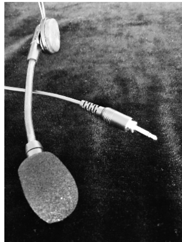
Figure 4: Dork-o-phone microphone in windscreen, 3.5mm mono plug. Photo by Carrie Rentschler, used with permission.
