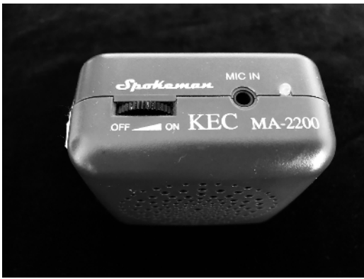
Figure 1: Dork-o-phone top view with power, LED and mic in. Photo by Carrie Rentschler, used with permission.
